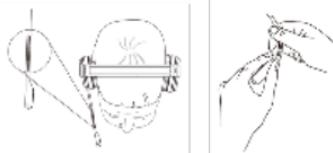
The Mono Space headset can be worn with the microphone on the left or on the right. Maintain the speaker firmly and rotate the boom arm by 180°. The maximum rotation angle is 270°.
