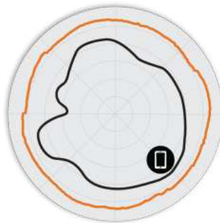
Figure 3. R750 5GHz AzimuthAntenna Patterns
