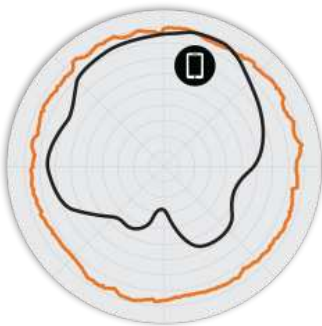
Figure 2. R750 2.4GHz AzimuthAntenna Patterns
